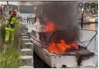
Since gas fumes are heavier than oxygen, they can settle at the bottom of the bilge where, if not completely ventilated, can easily be ignited by a spark from the engine or any part of your electrical system. That's why the **Sniff Test** is essential. Each year, there are needless fuel dock disasters where boats literally explode from fumes igniting. It's not a happy sight for the boat or its passengers.
